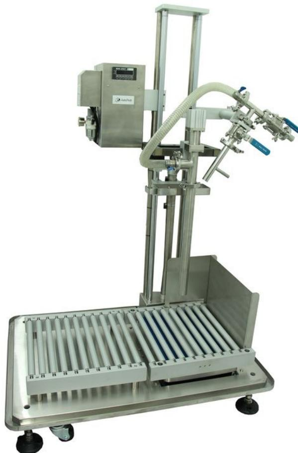
Weighing Filler is suitable for all kinds of High consistency, High viscosity, such as condensed milk, machine oil, shampoo, cosmetics and granule juice.
