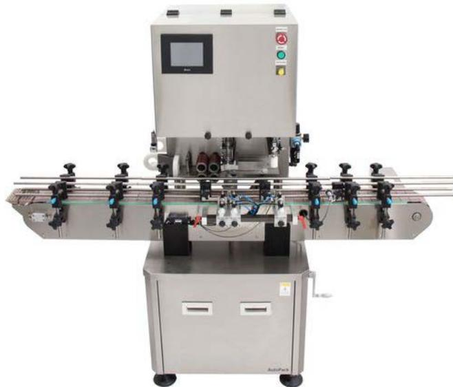
Automatic Cotton Inserter CI-415 applicable to the medicinal, health products, food industry. It can be inserted cotton into the container automatically.
