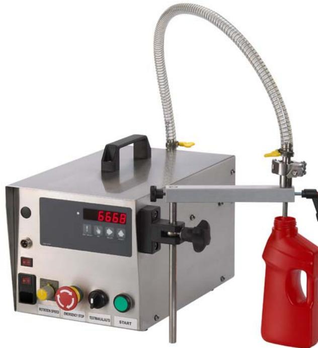
If you have large volume or high speed filling, Tabletop Gear Pump Liquid Filling Machine FG-100 is the best choice. It is able to achieve the output with 250ml per second by sophisticated module of gear pump and make the liquid filling to be best performance. FG-100 will satisfy your need for a relatively low volume, low cost, user friendly, high quality filling machine.
