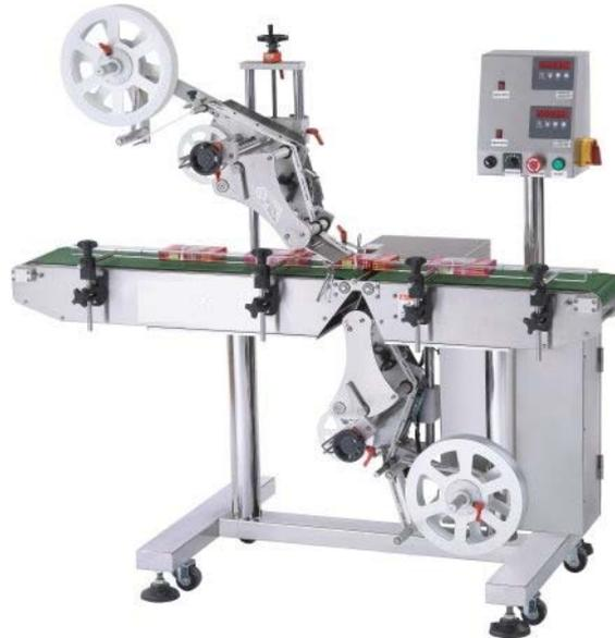
Automatic Top and Bottom Labeling Machine LTB-300 is high efficient labeling on top and bottom surface at one time.
